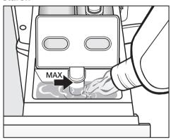
■ Load the fabric softener, shaper, or starch into compartment ※ . Do not exceed the maximum fill line.
